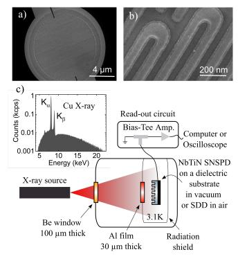
Fig. 1. (a,b) Scanning electron microscope images of the NbTiN detector revealing its structure: circular area with 10  $\mu$ m diameter, and 0.5 filling factor. (c) A diagram of the experimental setup. A copper X-ray source illuminates the NbTiN superconducting single photon detector (X-SNSPD) that is kept at cryogenic temperature of 3.1 K. The inset shows the corresponding X-ray spectrum.
