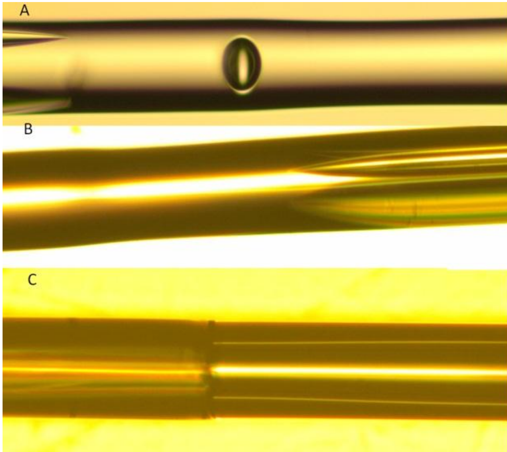
Figure 4.1: Micrographs showing: A) fusion done more than five times to THF and capillary junction, B) the fused capillary to THF with incorrect parameters, and C) an optimally fused THF to capillary assembly.
