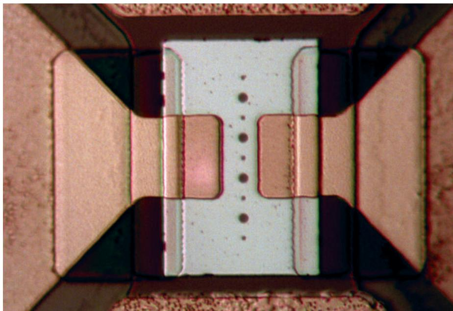
**Figure 1 |** Optical microscope image of the quantum-entangled LED developed by the team of researchers from Toshiba Europe and the University of Cambridge, UK.
